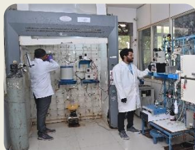
Vapor phase down flow quartz reactors
