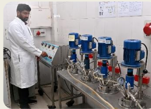
High pressure SS batch reactors
