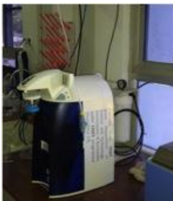
Type-1 Water Purification System
